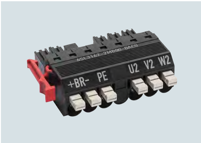
Power connector with push-in connection with snap-in actuators for Motor Modules, C/D type, 3 A to 30 A
